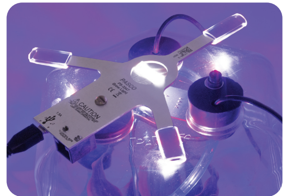
When connected to a //control.Node, the red and blue LEDs can be controlled using Blockly code, available in both SPARKvue and PASCO Capstone.
